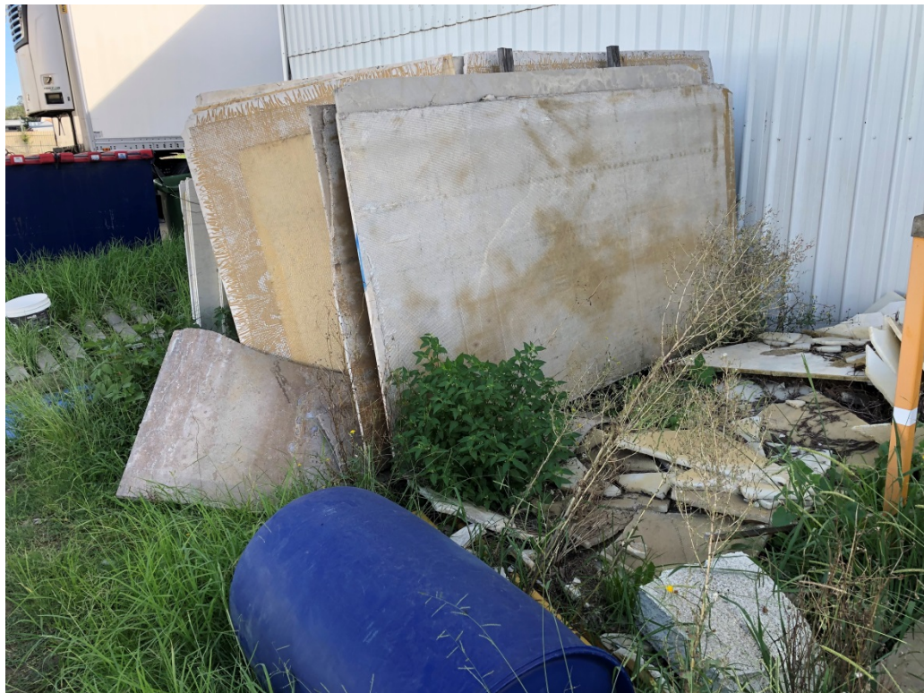
Photograph 12: Potential fibro-cement boards at the rear of the warehouse.
